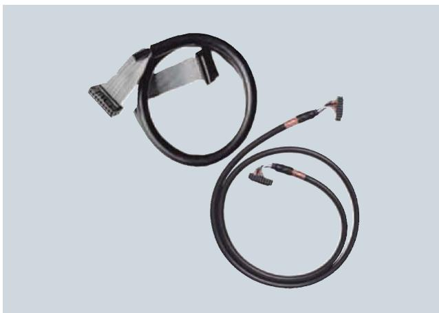
The connection cable is the linking element between the front connector module and the connection module. It transmits 8 signals and the supply voltage. The maximum bridgeable distance is 30 m. The connecting cable is available in two different versions:
